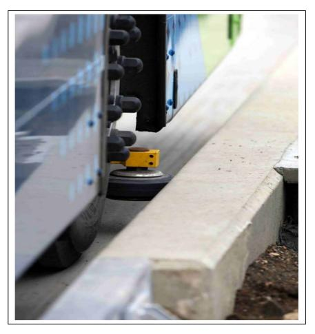
The photos above show: (top) a close up of a guide wheel, (bottom) a close up of the guide wheel running along the track.
