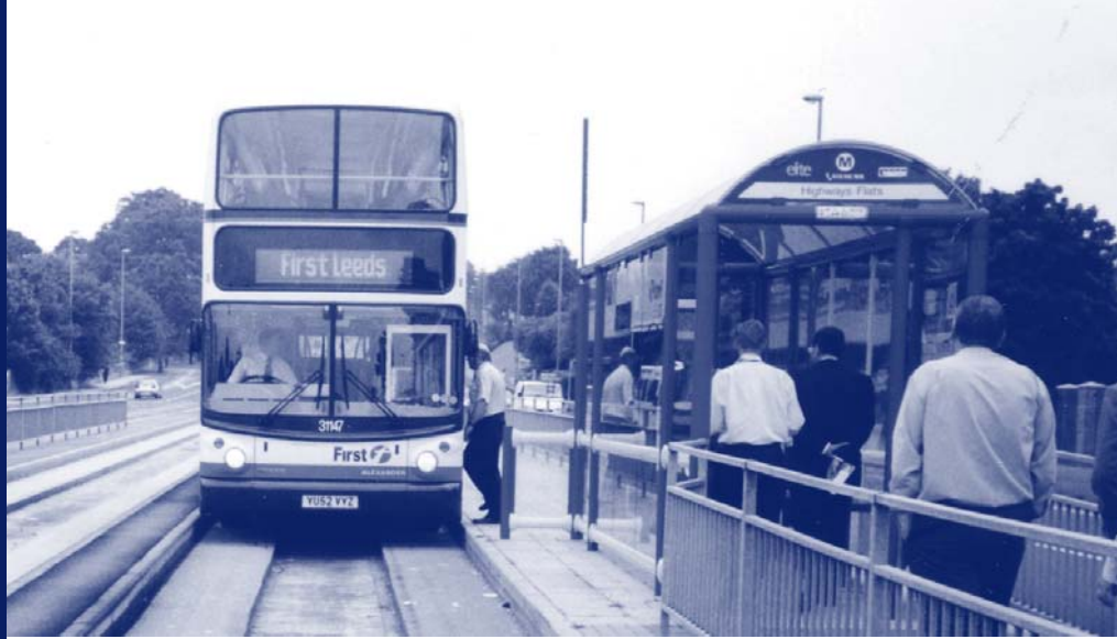
This photo shows a Guided Bus system which has been running in Leeds since 1994.
